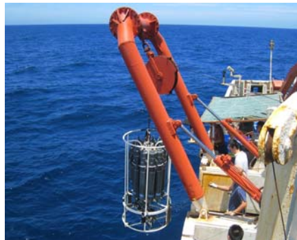
Students are getting the CTD off the ship. (Photo by Ying Liu)
