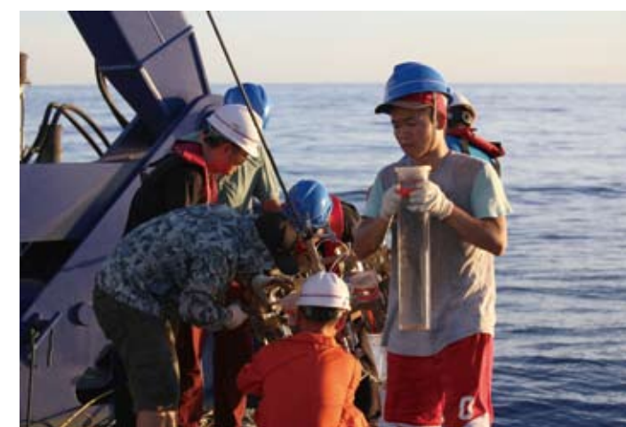
Scientists are retrieving the floating sediment trap in the SCS basin at the SEATS Station.
