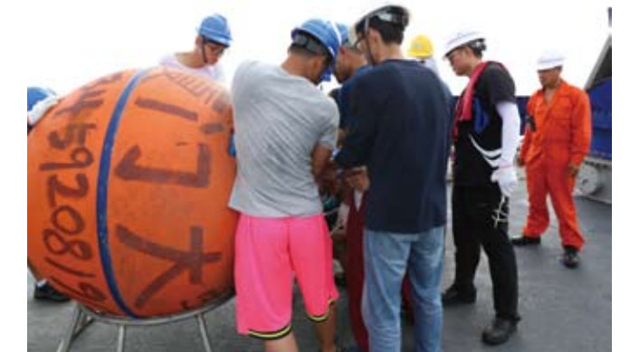
Subsurface moorings for the deep ocean were developed by Jianyu Hu and Zhenyu Sun's group to obtain stable and reliable data for long-term continuous observation in the South China Sea. It is MEL's first subsurface mooring at a deep basin. It was deployed in the middle-southern South China Sea by the R/V TTK in June 2017, and scheduled to be recovered in summer or fall 2018.
