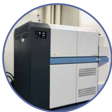
高分辨电感耦合等离子质谱仪 The high resolution inductively coupled plasma mass spectrometer (Element XR, Thermo Fisher Scientific)
