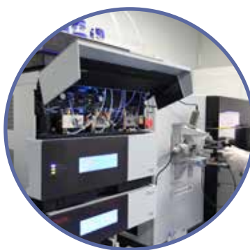
超高分辨率液相色谱—三合一质谱联用仪 Ultra high resolution liquid chromatography - tribrid mass spectrometer (Thermo Fisher UltiMate™ 3000 RSLCnano - Orbitrap Fusion™ Lumos™)
